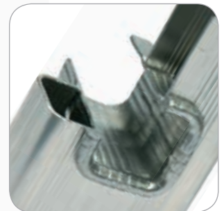
Stile/rung connection through triple expansion and crimping
