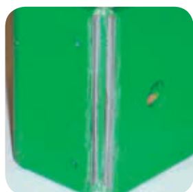
Steel parts coated with nylon
