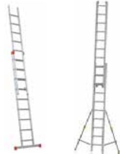
Introduction of stabilizing bars or stabilizers
