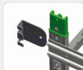
Fastening bracket: ladder and safety cage connection
