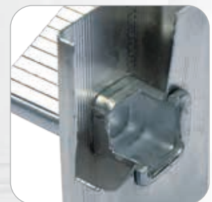
Stile/tread connection through triple expansion and crimping
